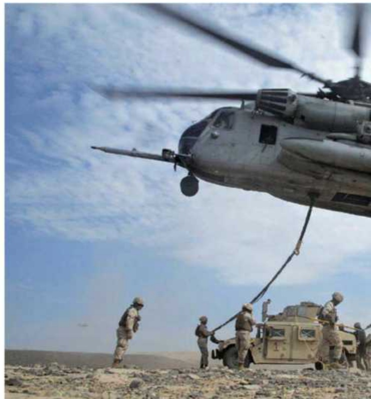
Marines use a CH-53E Super Stallion to lift a Humvee during an exercise at California's Camp Pendleton.
